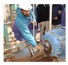
Precision alignment ensures the smooth, efficient transmission of power from the motor to the driven machine. Stresses inside a misaligned machine are caused when it to pulls against pipes, ducts, hold down bolts, etc. These stresses are transferred internally to rotors and stators causing more energy to be used to turn the motor.
