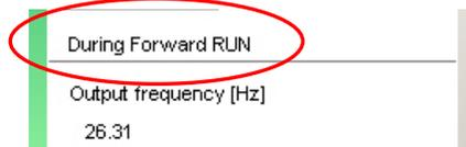
During run, a window will appear near the task tray to stopping the motor. When a Forward command is given, the icon will rotate counterclockwise.
