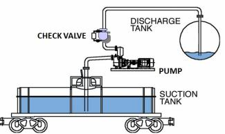
On start up the discharge was empty and the air could be purged. However, after the pumping cycle and the pump was stopped, the head of acid on the discharge check valve prevented the air from purging out on the priming cycle.
