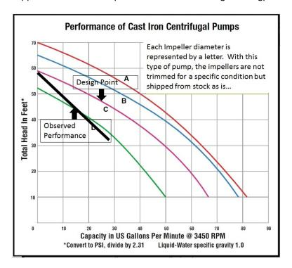
As you can see by the plot, the pump was not performing to spec.
