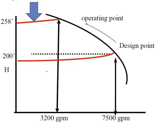
Minimum flow is 4500 gpm
