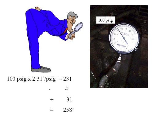
As you can see from the picture, the pump is running at 100 psig discharge pressure which is a head of 258', which means the pumps are operating at 3200 gpm which is below the pump's minimum flow of 4500 gpm. This was the reason for the failure of these pumps, and also the "poorly performing" original pumps.
