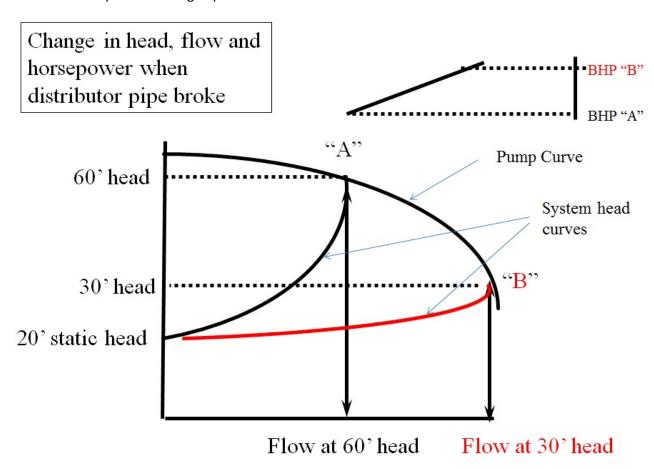
Without flow to the spray nozzles, the scrubbing liquid would "channel" through the packed column and it would lose its scrubbing efficiency.
