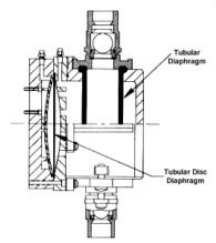
Hydraulically actuated pumps have one of two methods of control: amplitude modulation or hydraulic bypass. Hydraulically actuated amplitude modulation pumps operate in the same fashion their mechanically actuated counterparts: by varying stoke length.
