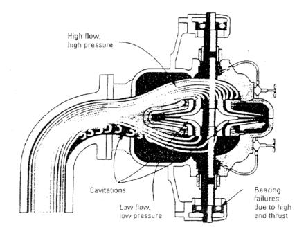
The out board end gets more flow due to the centrifugal force pushing the water to that side and the inboard side gets less flow. This creates flow instability and sometimes cavitation. Besides affecting performance, it will cause uneven pressure distribution and nullify the axial thrust balance of a double suction impeller. This will cause premature bearing failure due to excessive axial thrust.
