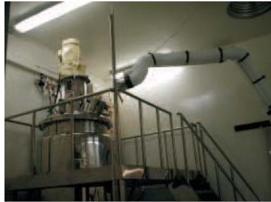
Poised for duty: a fume hood patiently awaits the opening of a reactor vessel containing hazardous materials.
