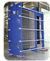
This newly assembled plate-and-frame heat exchanger can be unbolted, knocked down into individual pieces and reassembled on site.
