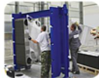
The list of tools required for typical maintenance work is a short one: a wrench, tape measure, and a set of gloves to protect your hands while handling the plates.
