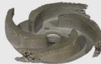
**Damage caused by discharge cavitation**
