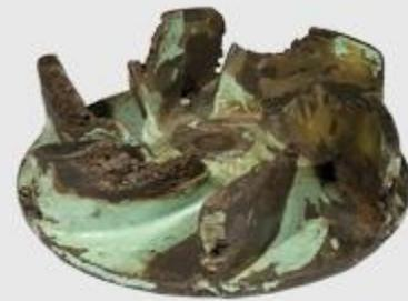
**Damage caused by both suction and discharge cavitation**
